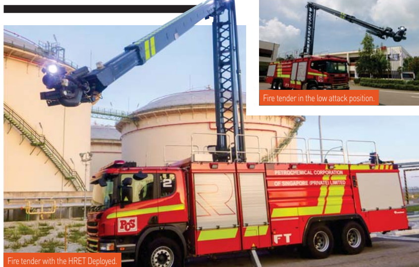
Fire tender with the HRET Deployed.
