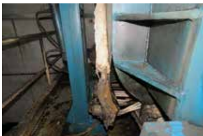
Deformed heating elements seen through the rupture on the oil jacket, rear of machine
